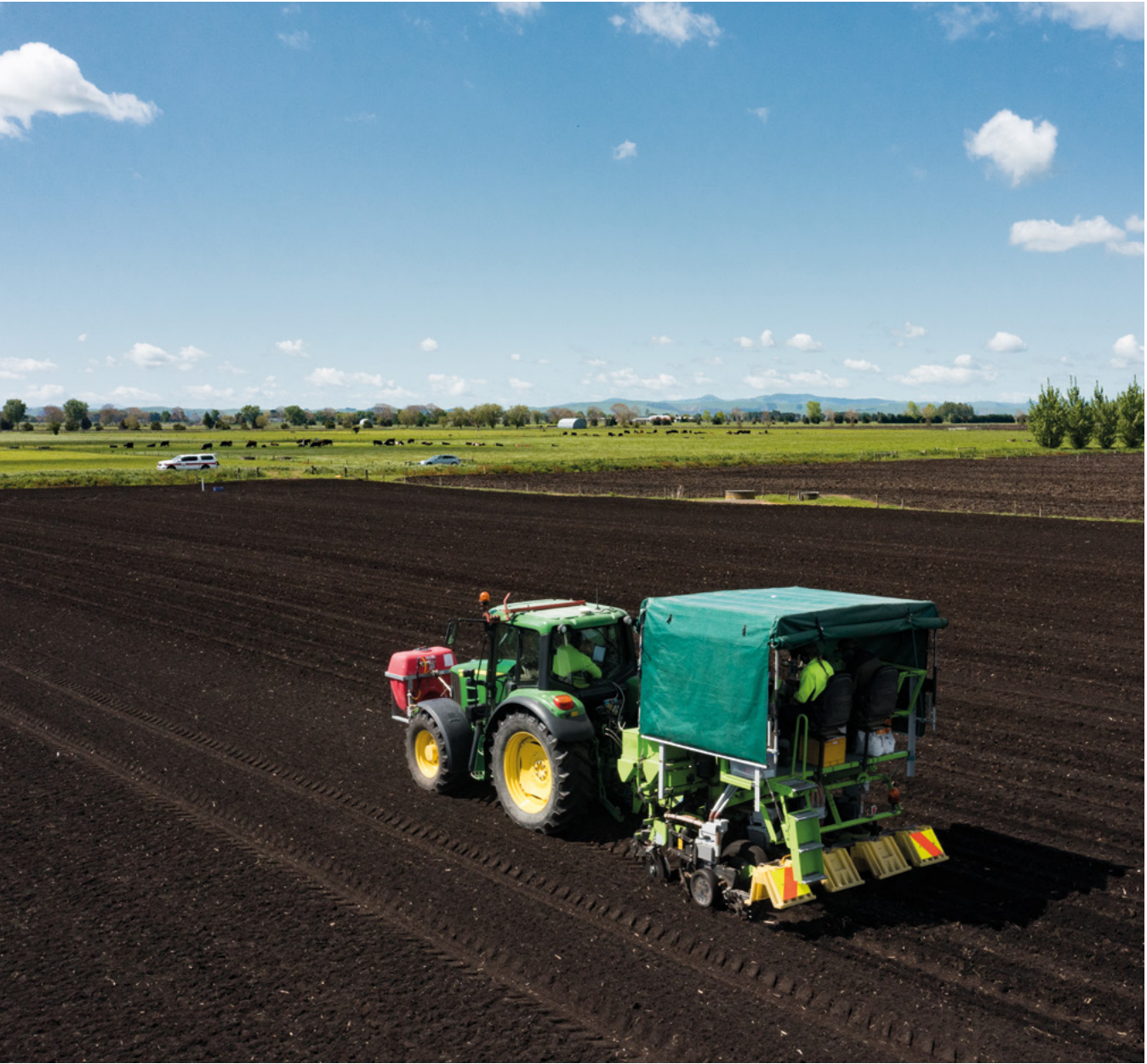
An IMPACT™ small plot planter at Gordonton, Waikato. IMPACT is the acronym for “intensively managed product advancement and characterisation trials”.
